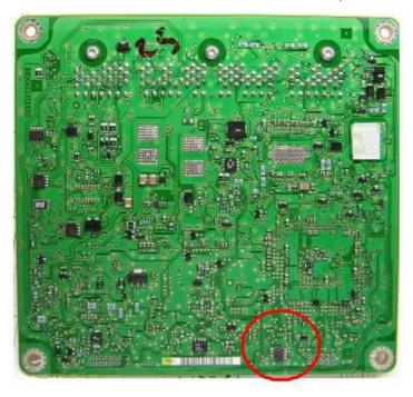
U'll identify the EEPROM by the numbers on the circuit board, which in most cases will be "**IC900**" and by the numbers on the top of the device itself, which will be any of following...au zingiine!
