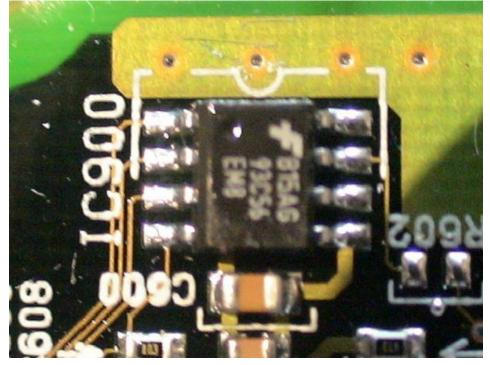
Alafu, U will require a capable Serial EEPROM programmer, yeyote, kwa mfano kama hii, lakini sio lazima hii....but can be any other that accepts serial EEPROMS of the **SPI**, **uWire** or **I2C** types. Some are expensive and some are not, but most will include protocols for handling such type of EEPROMs. A Windows software will be included on any of those Programmers for doing the job using your personal computer!
