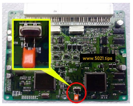
Hapo juu, we have an example of how to jump the crystal oscillator. It can be done with a piece of wire or like in the picture, with a capacitor of 1uf. If using a capacitor, the value is not critical as long as it is 1uf or more. Either the capacitor or jumper wire, must be soldered in parallel to the pins of the crystal.
