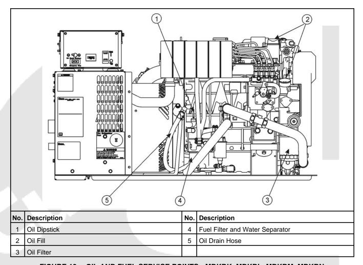
FIGURE 13. OIL AND FUEL SERVICE POINTS - MDKBK, MDKBL, MDKBM, MDKBN
