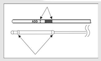
FIGURE 16. OIL LEVEL DIPSTICK ADD/FULL MARKINGS
