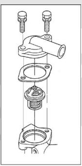
FIGURE 23. TYPICAL THERMOSTAT AND HOUSING
