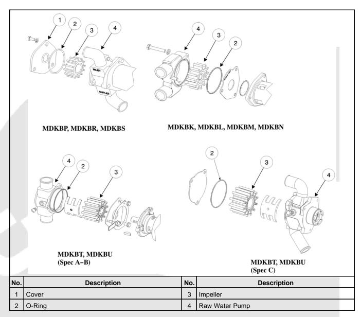
FIGURE 24. REPLACING THE RAW WATER PUMP IMPELLER
