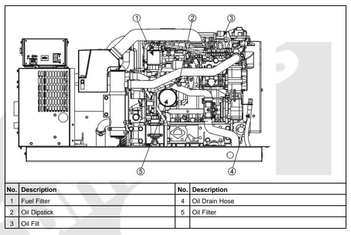
FIGURE 15. OIL AND FUEL SERVICE POINTS - MDKBT, MDKBU
