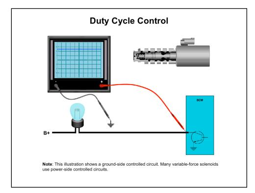
**Duty Cycle Control** The linear solenoid voltage is rapidly switched ON/OFF by the ECU. This creates a varying range of duty cycles between 0% and 100% based on the ratio of ON time to OFF time. This allows the solenoid to move to varying points between fully open and fully closed. The linear solenoid's spool valve has an infinite number of positions within its operating range.
