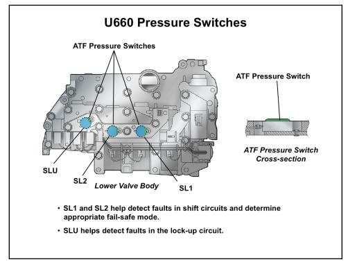
**U660 Pressure Switches** U660's ECU/TCM monitors three pressure switches to determine if the ECT is operating correctly. These are simple ON/OFF switches located in outlet passages from:
