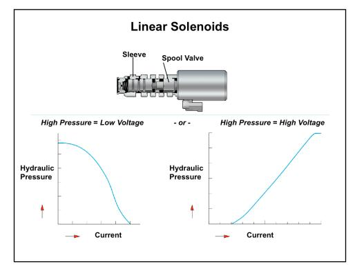
**Linear Solenoid** Linear solenoids are identified by an "SL" designation. They are typically connected to the electronic control circuit by two wires, because their ground is controlled through the ECU.
