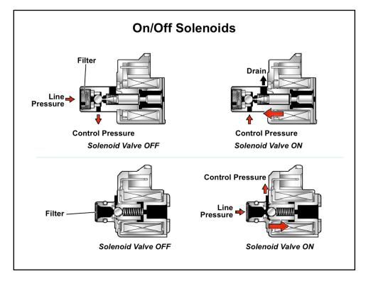
**ON/OFF Solenoid** ON/OFF solenoids are identified by an "S" designation. They are typically connected to the electronic control circuit by a single wire (the solenoid body provides the circuit ground). ON/OFF solenoids either receive voltage or no voltage, providing only two possible "duty cycles" — 0% or 100%.
