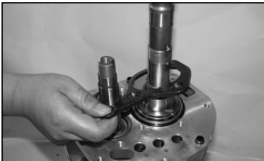
38. Remove the support axial lock plate
