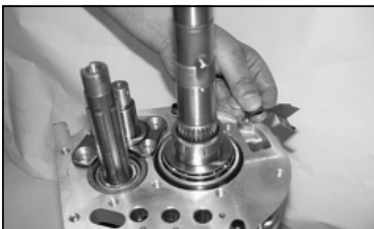
39. Remove the air duct grease baffle
