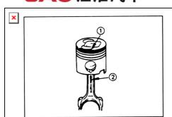
4) Install the piston onto the connecting rod.
