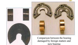
Foreign matters in the oil cause the bearing to be damaged
