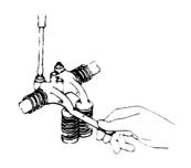
③ Check the clearance between intake valve and exhaust valve push rod for the first cylinder. If there is clearance between intake valve and exhaust valve push rod for the first cylinder, the first cylinder piston locates at the top dead center of compression stroke. If there is no clearance between intake valve and exhaust valve push rod for the first cylinder, the fourth cylinder piston locates at the top dead center of compression stroke.
