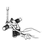
3 Check the clearance between intake valve and exhaust valve push rod for the first cylinder. If there is clearance between intake valve and exhaust valve push rod for the first cylinder, the first cylinder piston locates at the top dead center of compression stroke.
