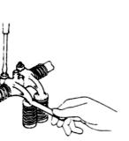
③ Check the clearance between intake valve and exhaust valve push rod for the first cylinder. If there is clearance between intake valve and exhaust valve push rod for the first cylinder, the first cylinder piston locates at the top dead center of compression stroke.
