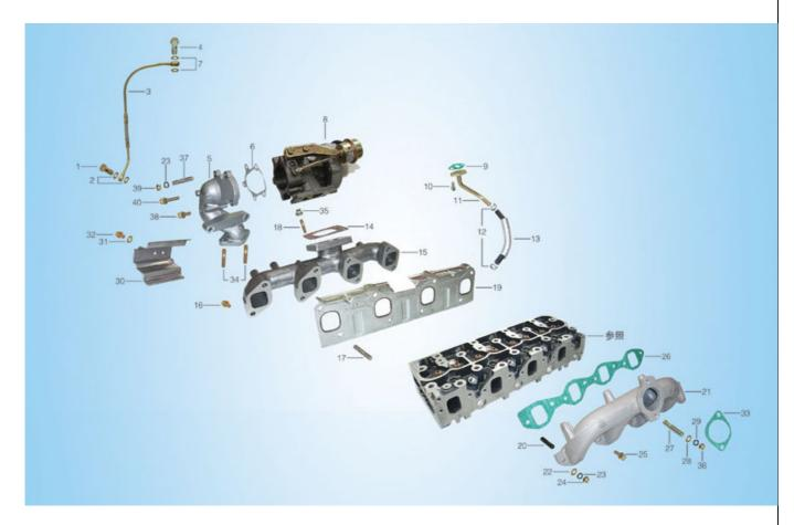
Engine intake/exhaust system mainly consists of air filter, intake pipe and exhaust pipe. If it is a supercharged engine, the system also includes the charger assembly. The installation and maintenance qualities may affect the engine performance and this factor has become particularly remarkable in the 4DA1-1 type chargers.
