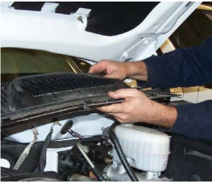
P24-4 To gain access to the motor, remove the shield cover from the cowl.
