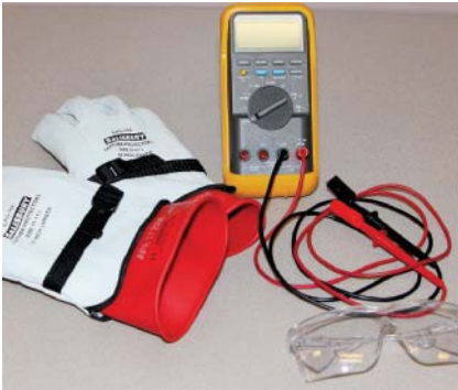
P2-1 Tools required to perform this procedure include safety goggles, 1000-volt-rated insulating gloves, and a digital multimeter (DMM).
