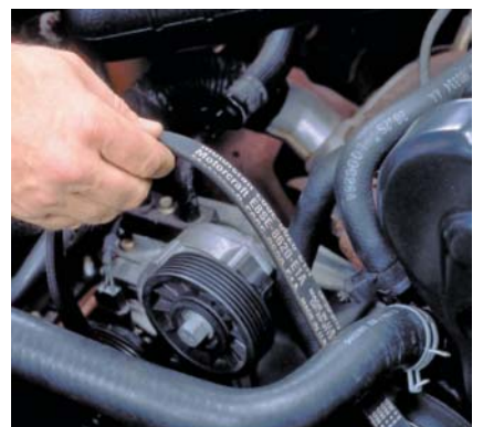
P13-9 Install the new belt over each of the pulleys following the recommended sequence.
