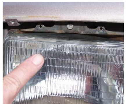
P15-9 Place the headlight into the shell assembly. When positioning the headlight, be sure that the embossed number is at the top. Many headlights are marked "TOP."
