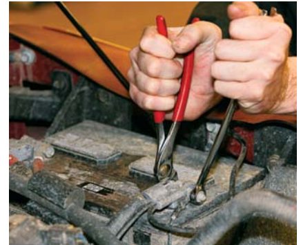
P9-3 Loosen the clamp bolt for the negative cable using terminal pliers and wrench of correct size. Be careful not to put excessive force against the terminal.
