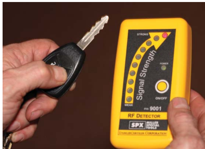
FIGURE 14-29 RF signal meter indicates the strength of the signal.
