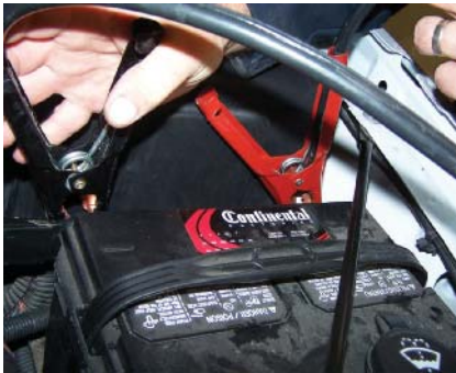
P18-7 After successful download, return to the vehicle and connect a battery charger to the vehicle's battery. Maintain about 13.5 volts on the battery.
