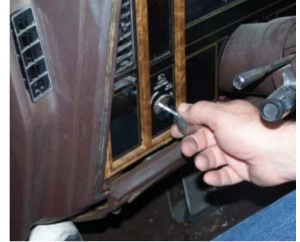
P15-12 Check operation of the headlight.
