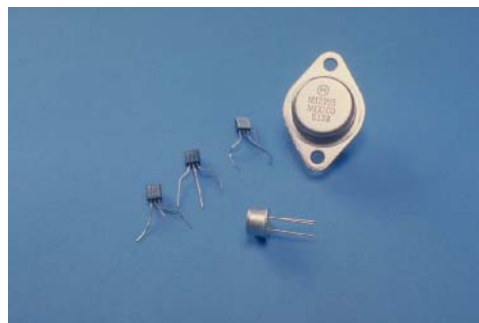
FIGURE 3-27 Transistors that are used in automotive applications.
