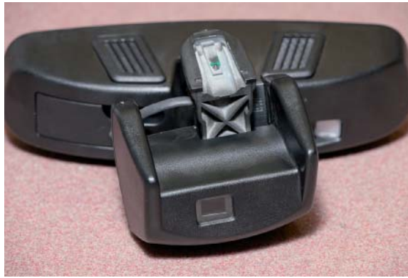
FIGURE 12-12 The SmartBeam auto headlight system uses a digital camera to determine oncoming light intensity.
