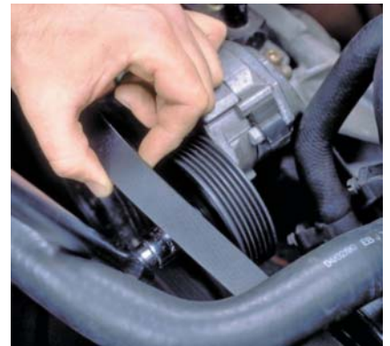
P13-6 Pry the idler pulley or generator to release the tension on the belt and remove the belt.
