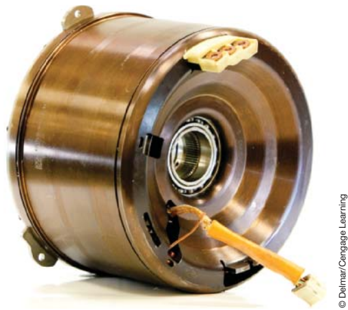
FIGURE 6-46 AC three-phase motor used in a HEV.
