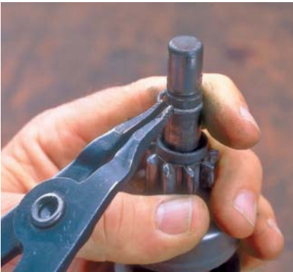
P10-13 Remove the snap ring.
