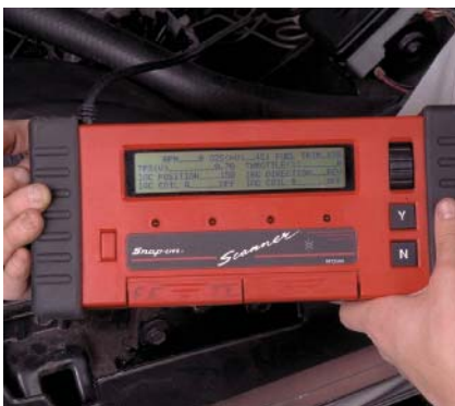
P17-7 Select the BODY function and retrieve the DTCs with the scan tester.
