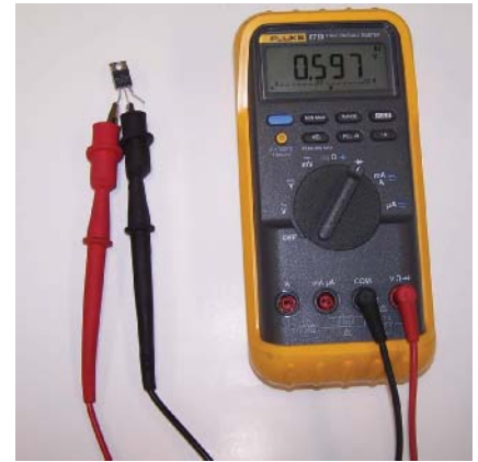
P5-3 If the positive probe is on the base of a good NPN transistor, you should read a low diode drop to pins 2 and 3. The base to collector diode drop will be slightly lower than the base to emitter reading.
