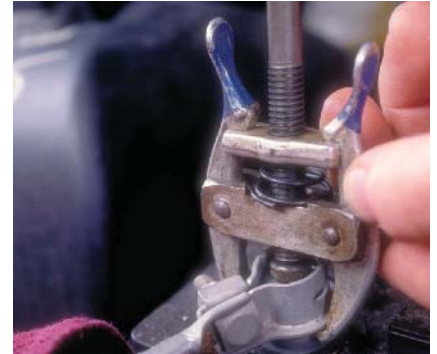
P16-3 Loosen the negative battery clamp bolt and remove the clamp using terminal pliers. Place the battery cable where it cannot contact the battery.
