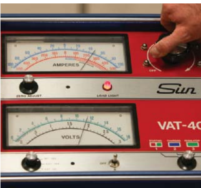
P8-7 Turn the load control knob slowly until the ammeter indicates the amperage amount determined in step 2.
