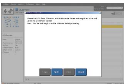
P30-7 When instructed, add the additional weight and follow the prompts to complete this phase. The scan tool should confirm the phase was completed successfully.
