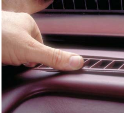
P21-11 Work the leading edge of the grill back into place using your thumb.
