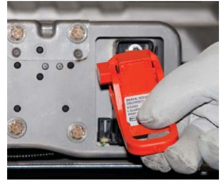
P2-6 Remove the high-voltage service plug and put it into your tool box or somewhere it cannot be accidentally reinstalled by someone else.
