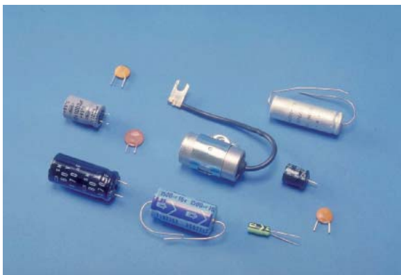
FIGURE 2-36 Capacitors that can be used in automotive electrical circuits.
