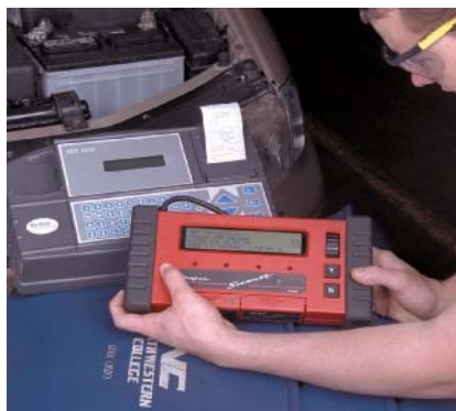
P17-8 Operate the system being diagnosed and obtain the input sensor and output actuator data with the scan tool.
