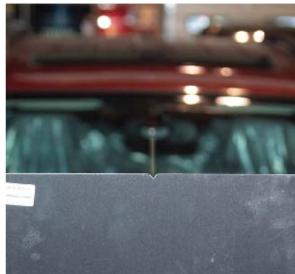
P22-14 While sighting through the V-notch in the upper edge of the calibration target, move the target left or right to align the target to the camera centerline marks on both the windshield and the rear glass.
