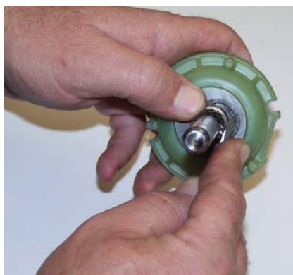
P11-8 Remove the lock ring from the output shaft and remove the stationary gear from the shaft.
