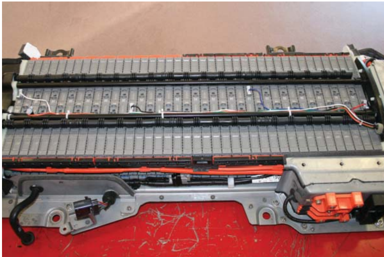
FIGURE 5-30 The modules of the HV battery.
