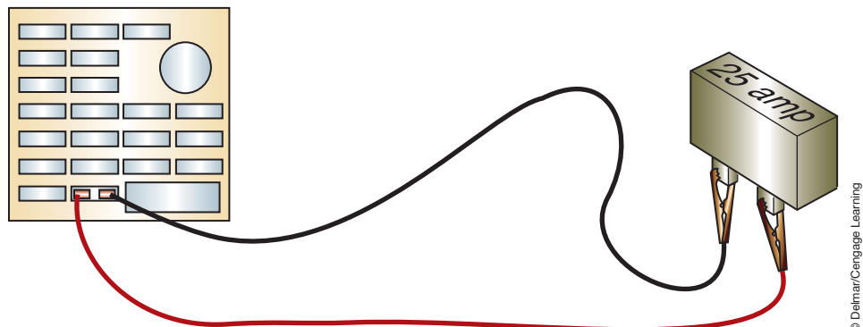
FIGURE 3-9 Use a circuit breaker to protect the circuit while checking for the short to ground.
