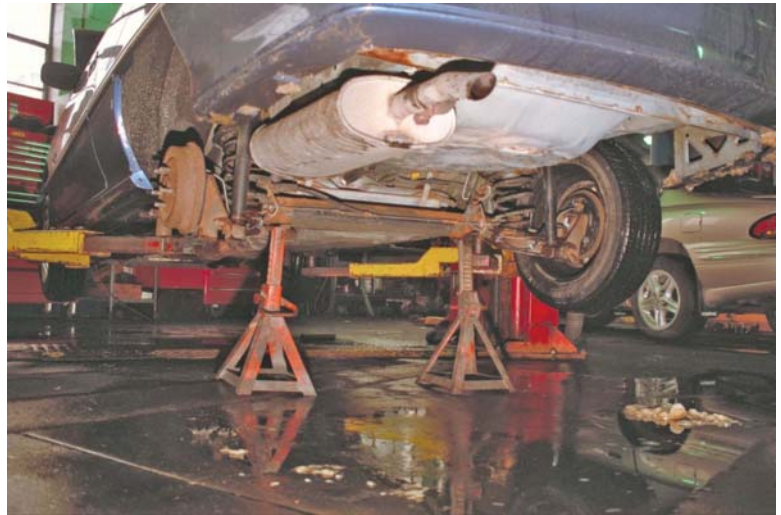
FIGURE 1-9 Support the vehicle by jack stands located at each corner that is lifted. Do not rely on the floor jack to support the vehicle.
