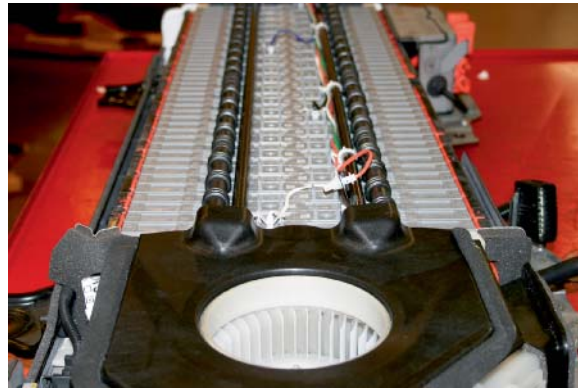
FIGURE 5-21 Battery pack made of several prismatic cells.
