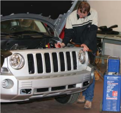
P8-1 Charge the battery to at least 75% and allow the battery to stabilize.
