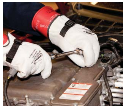
P2-8 After waiting at least 5 minutes for the high-voltage condenser inside the inverter to discharge, remove any covers necessary to access the isolation test locations.
