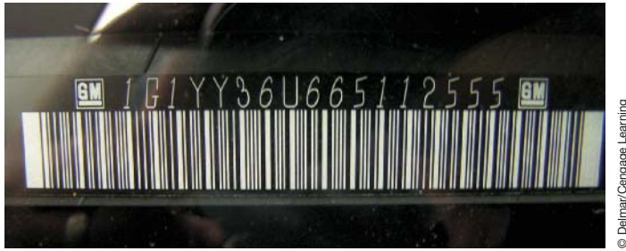
FIGURE 4-28 VIN plate location.
