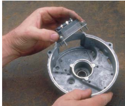
P14-11 Remove the rectifier bridge from the housing.
