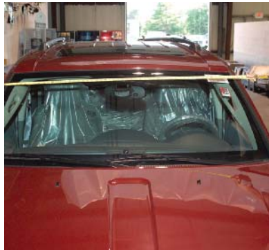
P22-2 Using the “ASI” marks on both sides of the windshield, measure across windshield using the shaft of the tint band arrow as the reference points.
