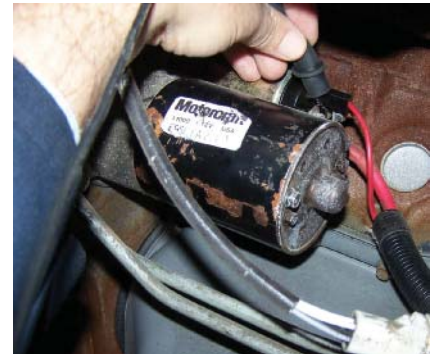
P4-3 Connect the negative lead of the meter to the main battery terminal on the starter motor.
