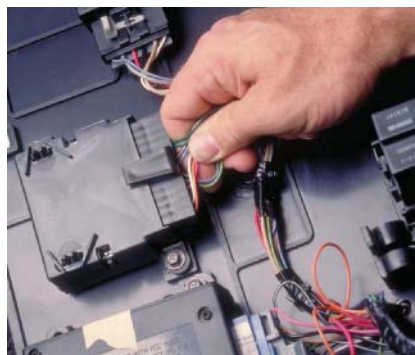
P27-8 Reconnect the relay harness.
