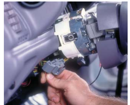
P16-9 Disconnect the turn signal switch electrical connectors.
