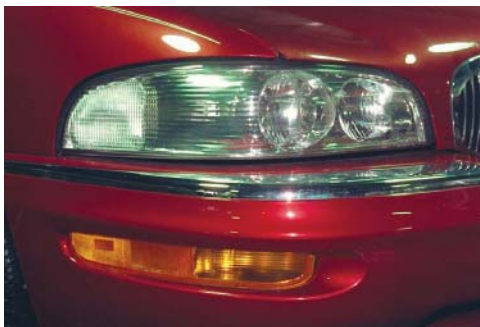
FIGURE 8-43 Wrap-around headlights serve as side marker lights.
