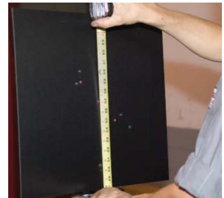
P22-15 Adjust the tripod so that the center LED on the target 57 inches (145 cm) from the floor.
