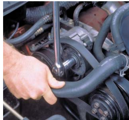
P13-5 If needed, loosen the mounting bracket bolt for idler or generator.
