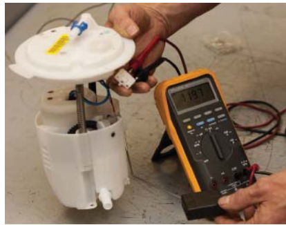
P23-5 Holding the sender unit in its normal position, place the float rod against the empty stop.
