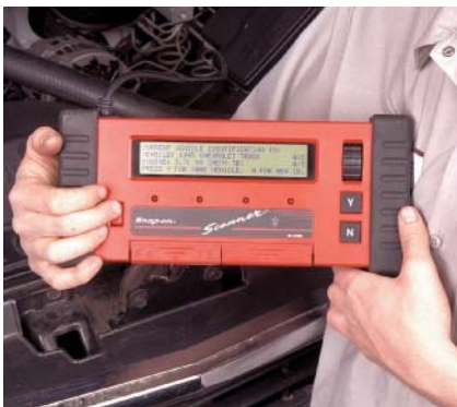
P17-4 Enter the model year and the VIN number code in the scan tester.
