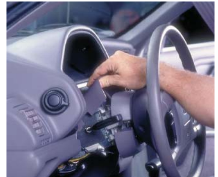
P16-6 Lower the steering column enough to remove the upper shroud.
