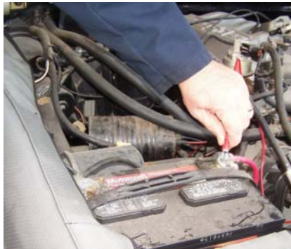
P4-2 Connect the positive lead of the meter to the positive battery post. If possible, do not connect the lead to the cable clamp.
