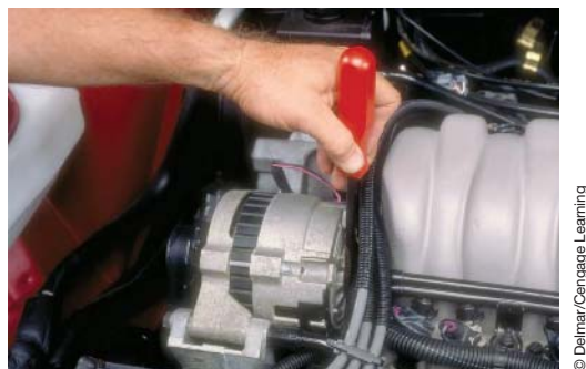
FIGURE 7-10 Quick check of the rotor and brushes.
