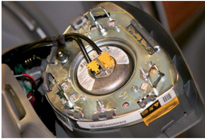
FIGURE 15-23 The multistage air bag module uses two squibs.
