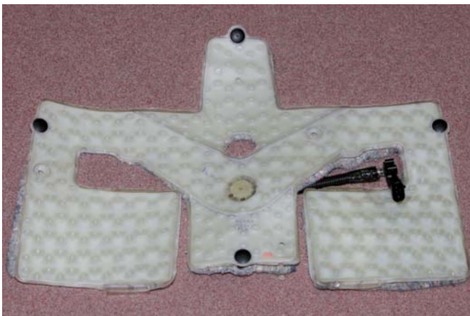
FIGURE 15-38 Bladder used to determine occupant classification.
