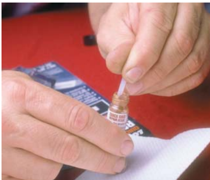
P26-4 Mix the hardener and silver plastic thoroughly. If the hardener has crystallized, immerse the packet in hot water.
