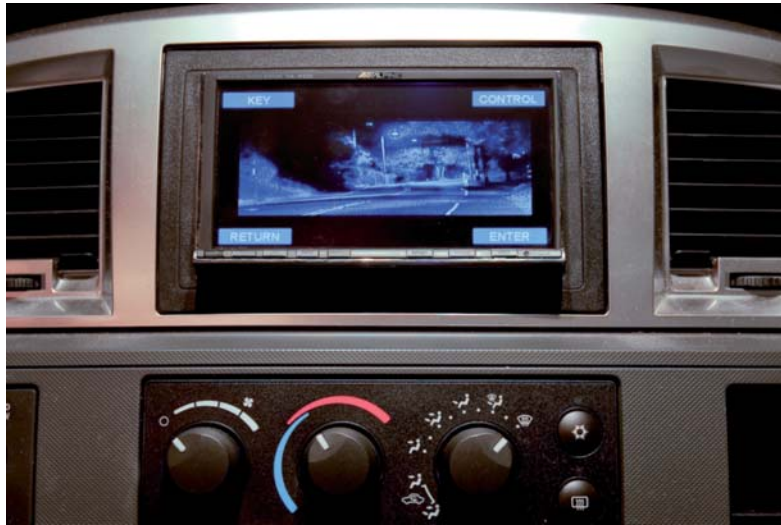
FIGURE 12-17 Night vision uses an infrared camera to project object onto a screen. The objects may be out of the range of the headlights.
