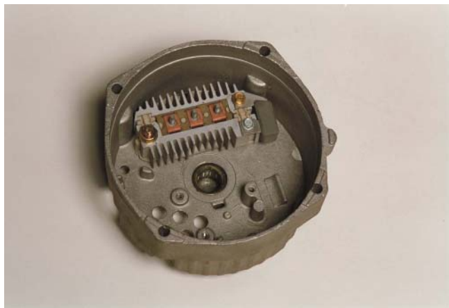
FIGURE 7-20 The positive-biased diodes are mounted into a heat sink to provide protection.
