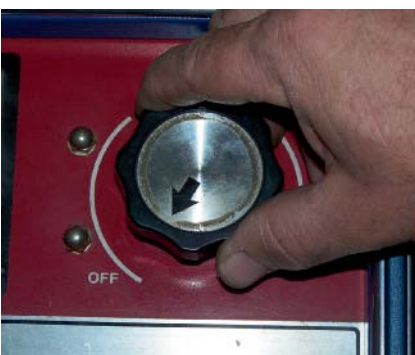
P12-8 Return the load control knob to the OFF position.
