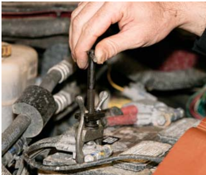
P9-4 Use the terminal puller to remove the cable from the terminal. Do not pry the cable off of the terminal.
