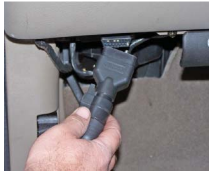
P18-8 Connect the scan tool to the DLC and power the tool on.
