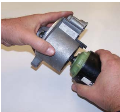
P11-4 Separate the drive end frame from the body. Remove the seal also.
