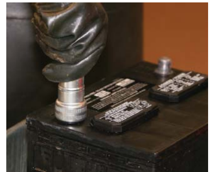
P9-15 Use the cleaning tool to clean the battery posts.
