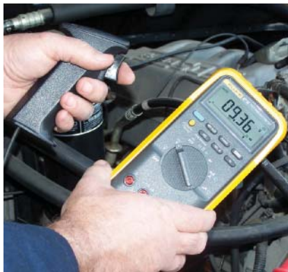
P4-5 With the engine cranking, read the voltmeter. The reading is the amount of voltage drop.
