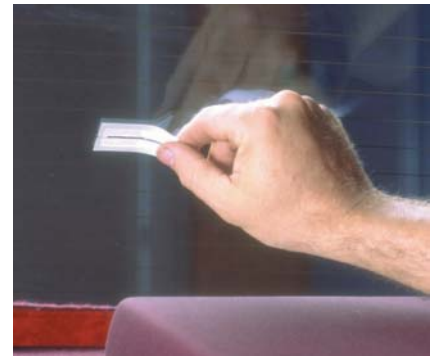
P26-3 Position a piece of tape above and below the grid. The tape is used to control the width of the repair.
