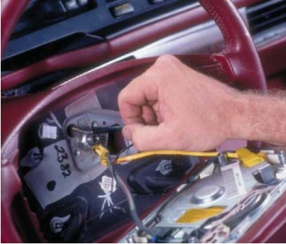
P29-10 Rotate the horn lead 1/4 turn and disconnect it.
