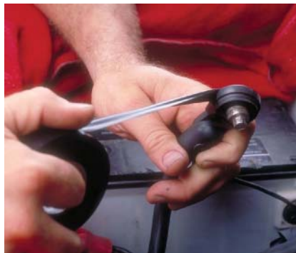
P29-5 Tape the cable terminal to prevent accidental connection with the battery post. Note: A piece of rubber hose can be substituted for the tape.
