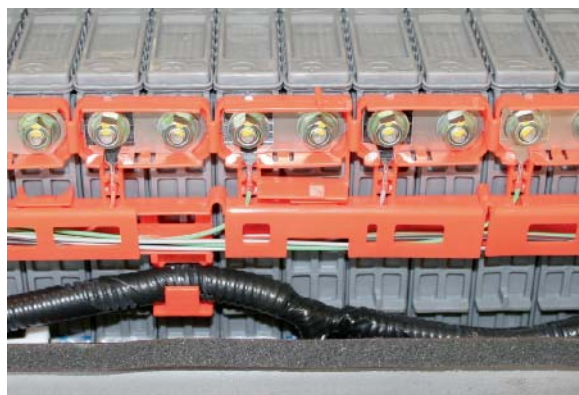
FIGURE 5-22 Cell module connections.
