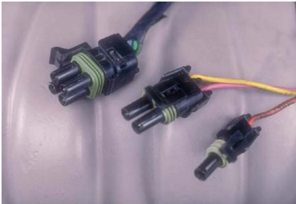
FIGURE 4-9 Weather-pack connector is used to prevent connector corrosion.
