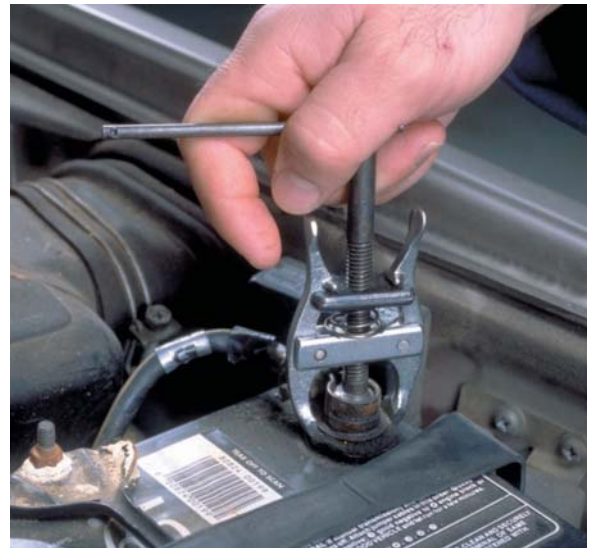
FIGURE 5-8 Use battery clamp pullers to remove the cable end from the terminal. Do not pry the clamp off.
