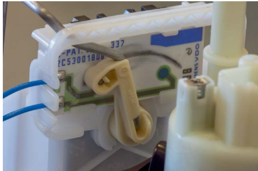
FIGURE 10-19 Magnetically coupled linear sensor used to measure fuel level.
