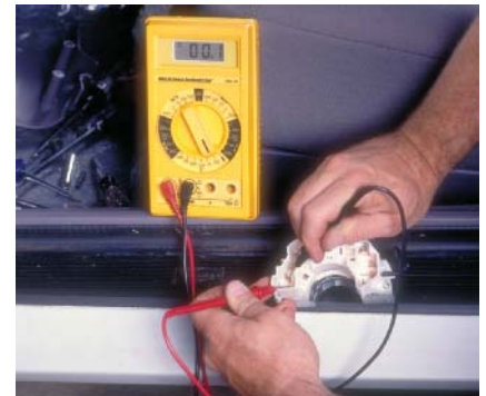
P16-15 With the switch in the high-beam position, continuity should be between terminals 15 and 12. Circuits 15 to 13, 196 to 13, and 196 to 12 should be open.
