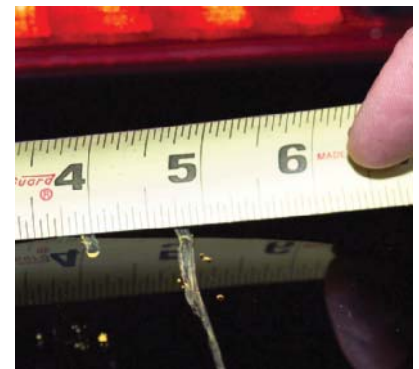
P22-9 Divide the upper measurement in half and mark that dimension on the glass using a grease pencil.
