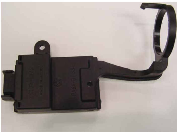
FIGURE 14-72 The immobilizer module with halo antenna.
