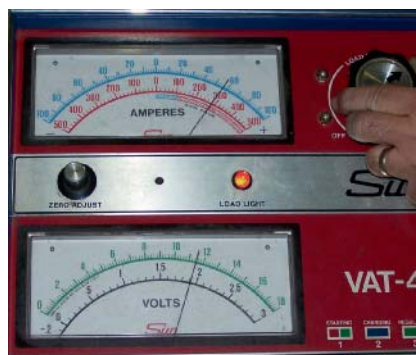
P12-7 Turn the load knob for the carbon pile slowly, until the highest ammeter reading possible is obtained. Do not reduce battery voltage below 12 volts.
