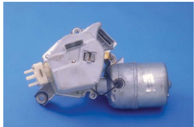
FIGURE 14-29 General Motors' pulse-type washer system incorporates the washer motor into the wiper motor.
