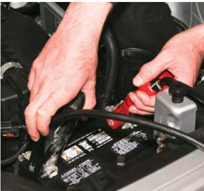
P8-4 Connect the large load leads across the battery terminals, observing polarity.
