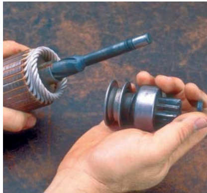
P10-14 Remove the retainer from the shaft and remove the clutch and spring from the shaft. Press out the drive housing bushing and the end frame bushing.
