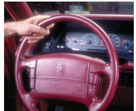
P29-3 Place the front wheels in the straight ahead position and turn the ignition switch to the lock position.
