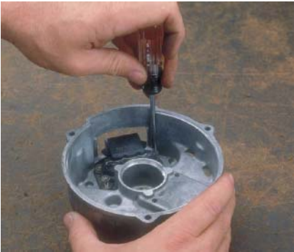
P14-10 Using a T20 TORX, remove the four attaching bolts that hold the rectifier bridge.
