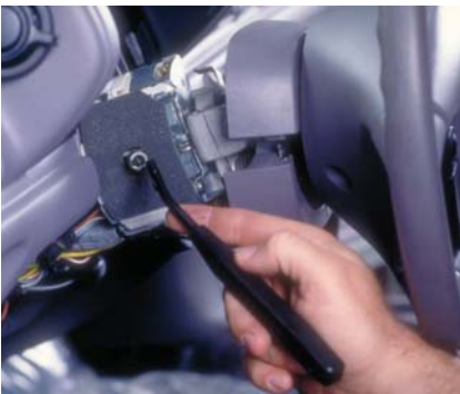
P16-7 Remove the turn signal lever by slightly rotating the outer end of the lever then pulling straight out on the lever. Some levers may be attached with fasteners.
