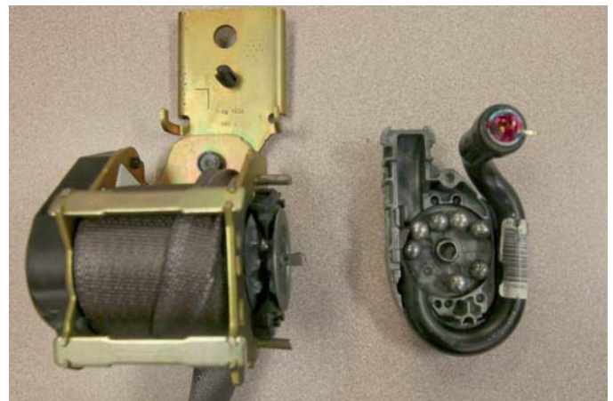
FIGURE 15-35 The balls are shot at the fan wheel, which causes the retractor to wind up the seatbelt tight against the occupant.
