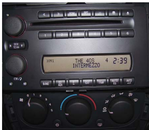
FIGURE 14-101 Satellite radio system.
