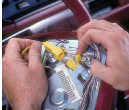
P29-11 Disconnect the electrical connectors.
