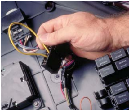
P27-4 Move the jumper wire to connect terminals D and C.
