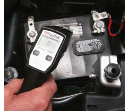
P8-3 Determine the temperature of the electrolyte. If the case is sealed, measure the temperature of the case.
