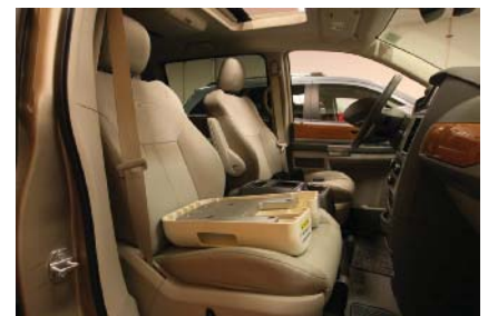
P30-6 When instructed, add the correct weight amount to the seat. Follow the scan tool prompts to complete this phase of the process. The scan tool should confirm the phase was completed successfully.
