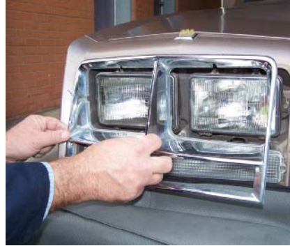
P15-11 Install the headlight bezel.
