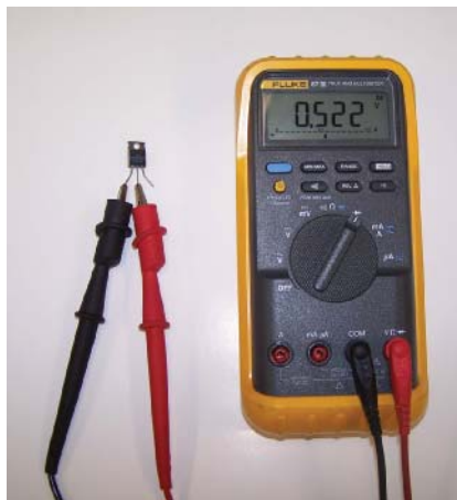
P5-5 If the reading is high when all three pins are tested, repeat the tests with the negative probe as the common pin. A pair of low readings now indicates a PNP transistor.
