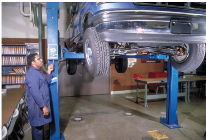
FIGURE 1-13 One type of hoist that may be used in the automotive shop. The hoist is used to raise the entire vehicle.
