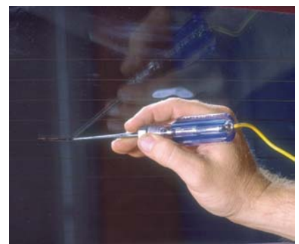
P26-9 Test the repair with a test light. Note: It takes 24 hours for the repair to fully cure.
