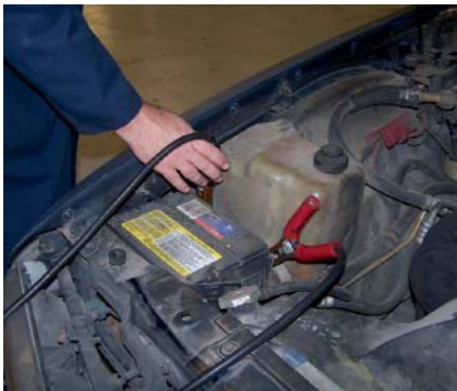
P12-1 Connect the large red and black cables across the battery, observing polarity.
