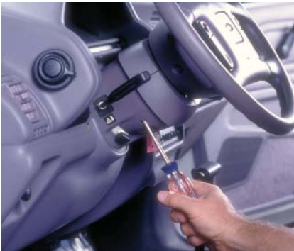
P16-4 Remove the shroud retaining screws and remove the lower shroud from the column.
