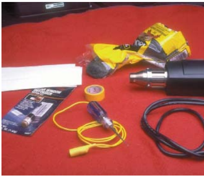
P26-1 Tools required to perform this task include masking tape, repair kit, 500°F heat gun, test light, steel wool, alcohol, and a clean cloth.
