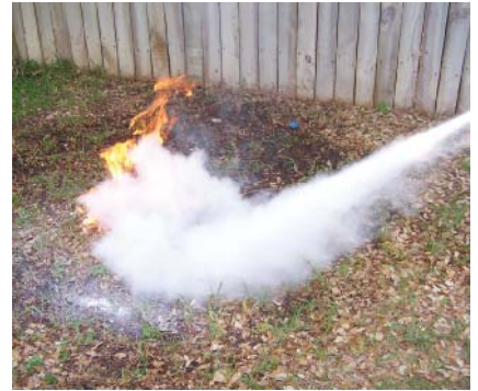
P1-6 Squeeze the lever while sweeping the hose from side to side. Keep the hose aimed at the base of the fire.
