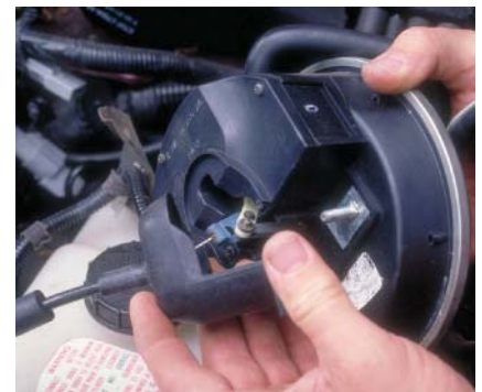
P28-9 Remove the two cable cover to servo assembly retaining bolt and pull off the cover.
