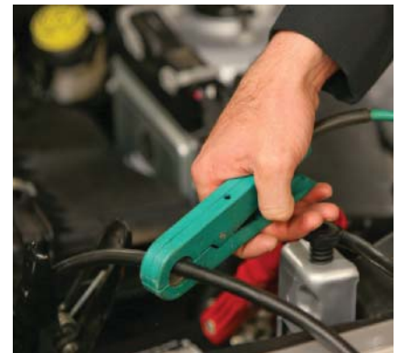
P8-6 Connect the ammeter's inductive pick-up around the negative load tester lead (not the battery's negative cable).
