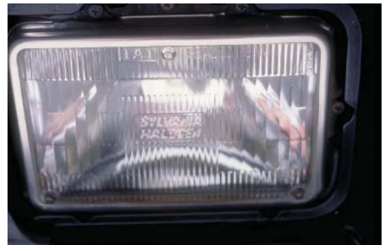
FIGURE 8-4 The lens uses prisms to redirect the light.
