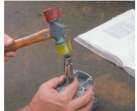
P14-12 Use a socket to tap out the bearing from the housing.
