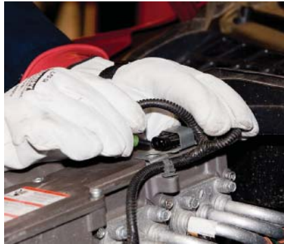
P2-5 If equipped, disconnect the 12-volt in-line connector to isolate the 12-volt battery. If the vehicle does not have the in-line connector, disconnect the negative (-) terminal of the auxiliary (12-volt) battery. Always disconnect the auxiliary battery prior to removing the high-voltage service plug.
