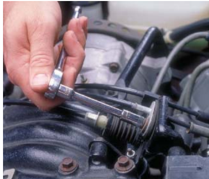
P28-2 Remove the retaining screws attaching the speed control actuator cable to the accelerator cable bracket and intake manifold support bracket.
