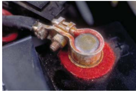
FIGURE 5-27 A protective pad under the battery clamp prevents corrosion of the clamp and terminal.
