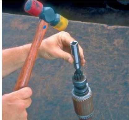
P10-11 Place a 5/8" deep socket over the armature shaft until it contacts the retaining ring of the starter drive.
