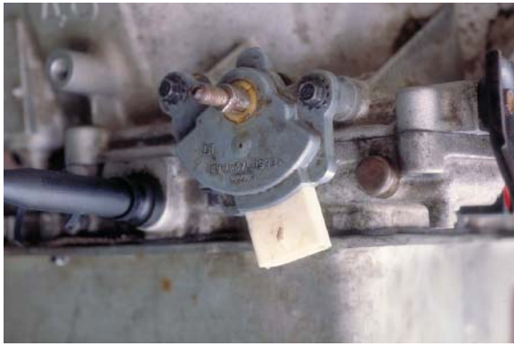
FIGURE 6-36 The neutral safety switch can be combined with the backup light switch and installed on the transmission case.
