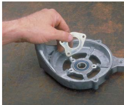
P14-17 Remove the bearing retainer.
