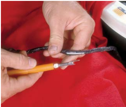
P6-4 If the wiring harness is taped, use a seam ripper to open the wiring harness.
