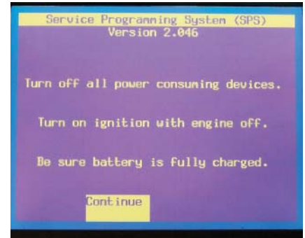
P18-9 Navigate the scan tool to perform the desired flash. Follow the instructions that are displayed on the screen.
