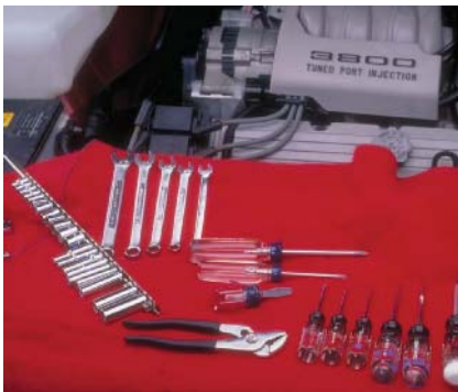
P29-1 Tools required to remove the air bag module include safety glasses, seat covers, screw driver set, torx driver set battery terminal pullers, battery pliers assorted wrenches, ratchet and socket set, and service information.
