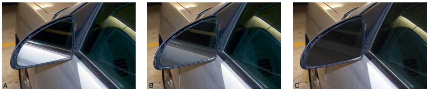
FIGURE 14-42 Electrochromic mirror operation (A) Day time; (B) Mild glare; (C) High glare.
