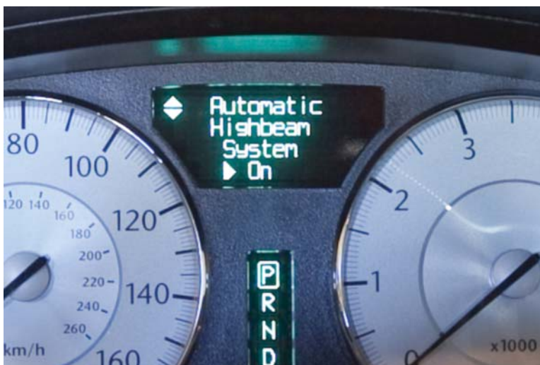
FIGURE 12-6 For the auto high-beam function to operate, it must be activated.
