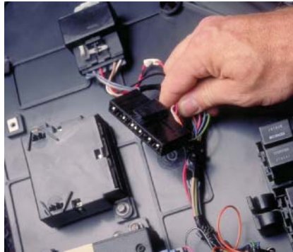
P27-2 Disconnect the relay wiring harness.
