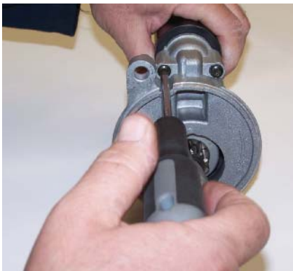
P11-1 Disconnect the lead to the field coil and remove the solenoid retainer screws.
