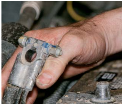
P9-5 Locate the negative cable away from the battery.
