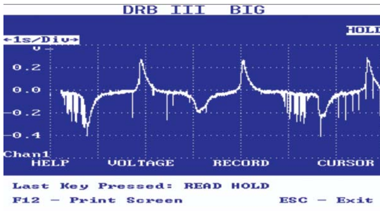
FIGURE 7-24 Waveform indicating an open diode in the diode trio.
