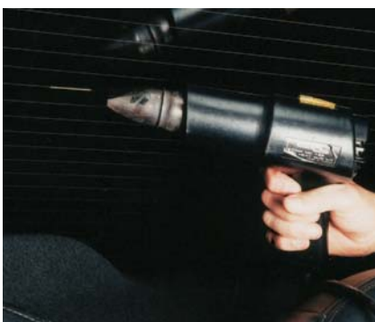
P26-7 Apply heat to the repair area for 2 minutes. Hold heat gun 1" (25 mm) from the repair.
