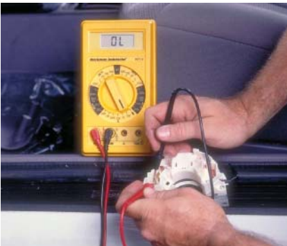
P16-13 With the switch in the low-beam position, the circuit should be open between terminals 15 and 12.
