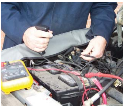
P4-7 Crank the engine and touch the negative test lead to the starter side of the relay. Observe the voltmeter while the engine is cranking.
