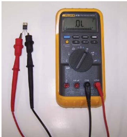
P5-4 If one or both measurements to pins 2 and 3 is/are high, put the positive probe on pin 2 and retest. If still high, put the positive probe on pin 3 and retest.
