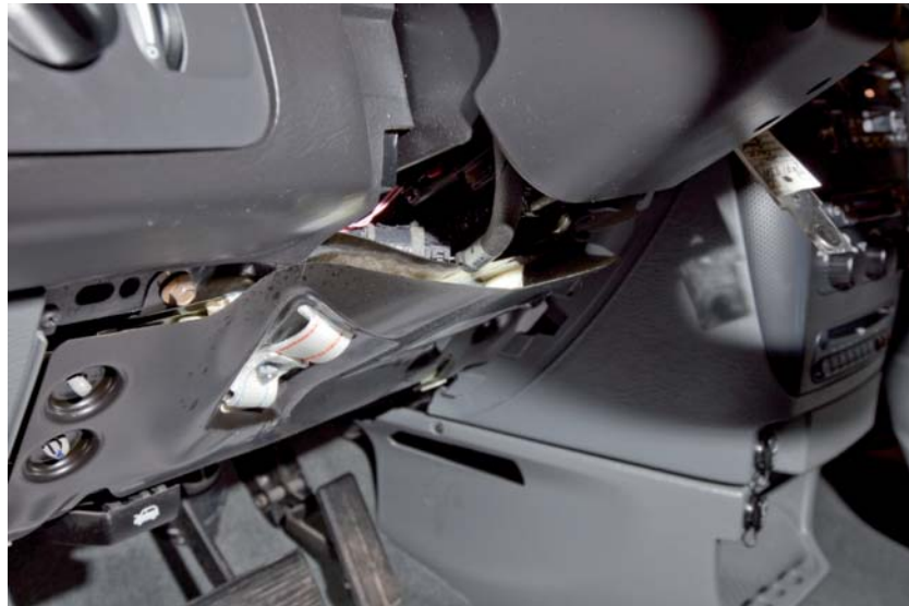
FIGURE 15-36 Inflatable knee blocker.
