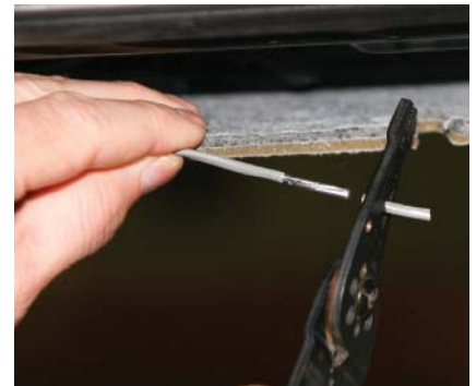
PS7-3 Being careful not to cut into the Mylar tape or to cut the drain wire, remove about 1 inch (25mm) of the outer jacket from the ends of each cable.
