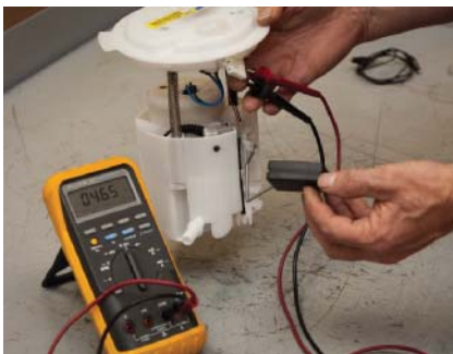
P23-7 Slowly move the float toward the full stop while observing the ohmmeter. The resistance change should be smooth and consistent.
