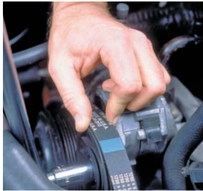
P13-11 Confirm that the belt is properly located into each pulley.
