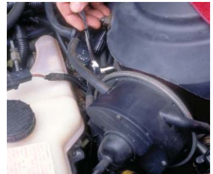
P28-6 Remove the two retaining bolts that attach the servo assembly bracket to the shock tower.
