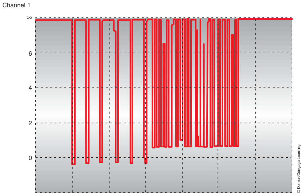
FIGURE 11-3 ISO K data bus transmission voltages.
