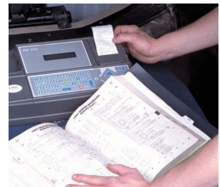
P17-9 Compare the input sensor and output actuator data to specifications in the appropriate service information. Determine data that is not written specifications.
