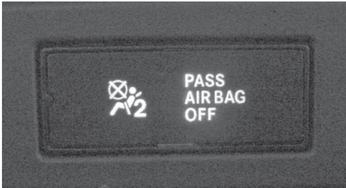
FIGURE 15-37 The PADL illuminates if the air bag is suppressed.
