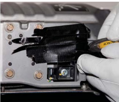
P2-7 Cover the high-voltage service plug receptacle with insulation tape.
