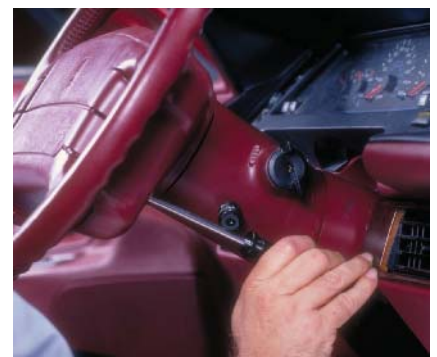
P29-9 Remove the four bolts that secure the module from the rear of the steering wheel.
