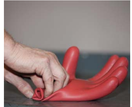
P2-3 Test the integrity of the insulating gloves prior to use. Wear the gloves until the high-voltage isolation procedure is complete.
