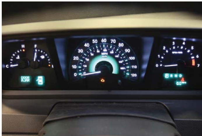
FIGURE 13-10 Electronically controlled swing needle instrumentation.
