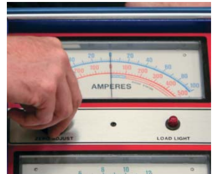
P12-3 Zero the ammeter.
