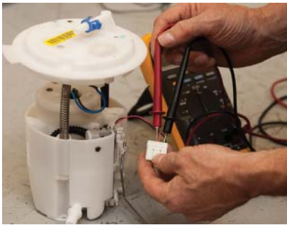
P23-4 Connect the positive test lead to the variable resistor terminal.
