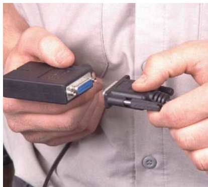
P17-5 Select the proper scan tool data cable for the vehicle being tested.
