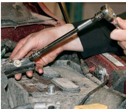
P9-7 Disconnect the hold down fixture.
