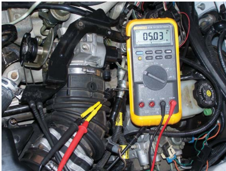
FIGURE 3-31 It may be necessary to use jumper wires to connect the wire connector to the sensor in order to measure voltage.
