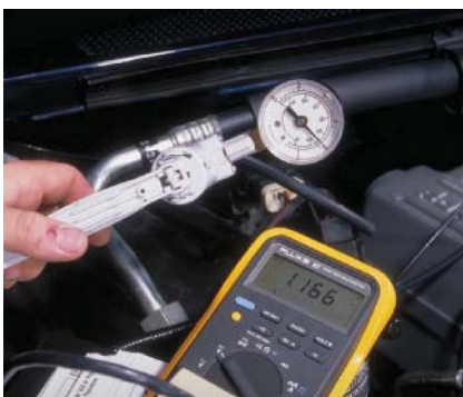
P19-7 Increase the vacuum applied to the MAP sensor to 10 in. Hg and observe the reading. Compare this reading to specifications.
