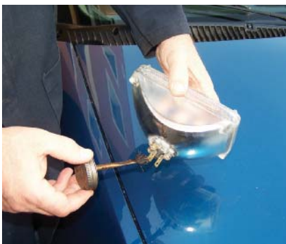
P15-7 Coat the connector terminals and the prongs of the new headlight with dielectric grease to prevent corrosion.
