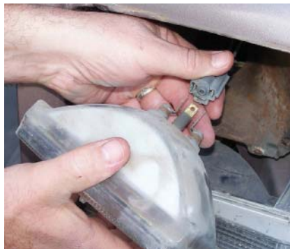
P15-5 Disconnect the wire connector from the back of the lamp.
