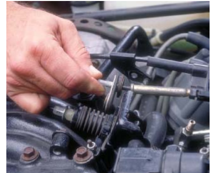
P28-3 Disconnect the cable from the brackets.
