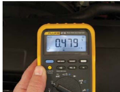
P3-5 Turn on the headlights (low beam) and observe the voltmeter readings. The voltmeter will indicate the amount of voltage that is dropped between the battery and the headlight.
