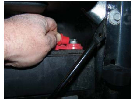
P3-3 To test the voltage drop of the whole insulated side of the circuit, connect the red (positive) voltmeter test lead to the battery positive (+) terminal.
