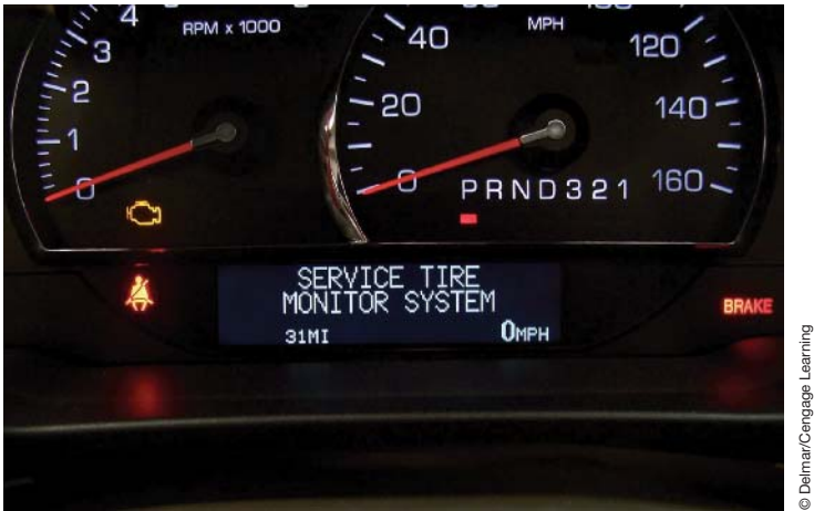
FIGURE 12-30 The computer-driven vehicle information center keeps the driver aware of the condition of monitored systems.
