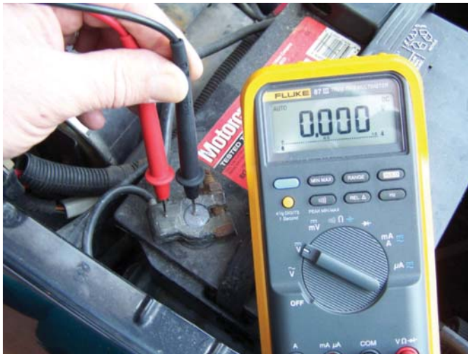
FIGURE 5-7 Voltmeter connections for the battery terminal test.
