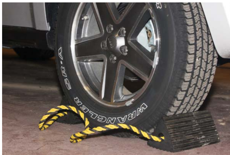
FIGURE 1-10 Before lifting the vehicle with floor jacks, block the wheels to prevent them from rolling.
