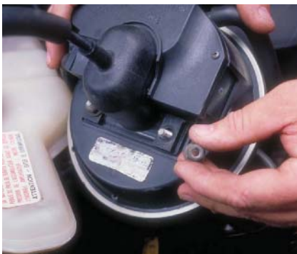
P28-7 Remove the two bolts that attach the servo assembly to the bracket.
