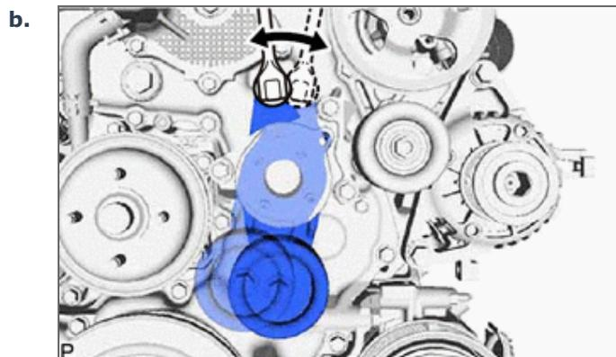
Check that nothing gets caught in the V-ribbed belt tensioner assembly by turning it clockwise and counterclockwise.
