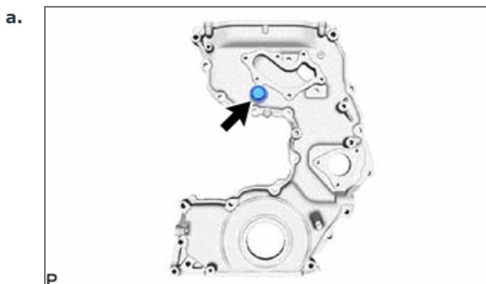
Remove the oil pump relief valve plug and gasket from the timing chain cover sub-assembly.
