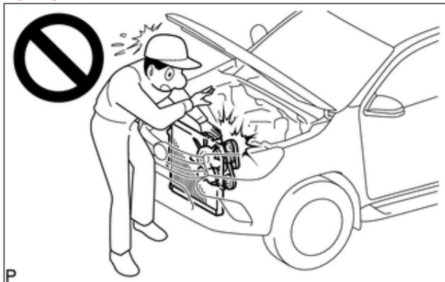
To prevent injury due to contact with an operating fan and generator V belt or cooling fan, keep your hands and clothing away from the fan and generator V belt and cooling fans when working in the engine compartment with the engine running.
