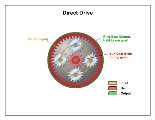
**Direct Drive** When any two members are held together and another member provides the input turning force, the entire assembly turns at the same speed as the input member.
