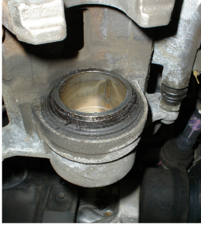
Example of Leaking Caliper Piston
