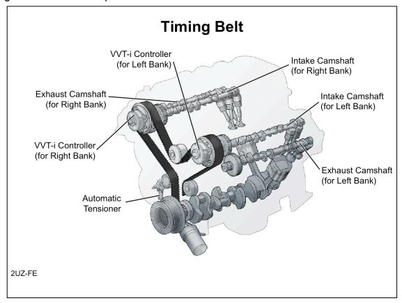
**Timing Belt** A timing belt performs the same function as a timing chain; it's just made of a different material. A timing belt is "toothed" so that it doesn't slip, an event which would clearly alter engine timing and performance.
