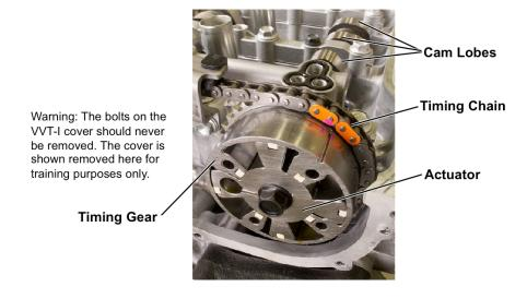
**VVT-i** Under some load conditions, the engine operates more efficiently if the exhaust valve closes before the intake valve opens.
