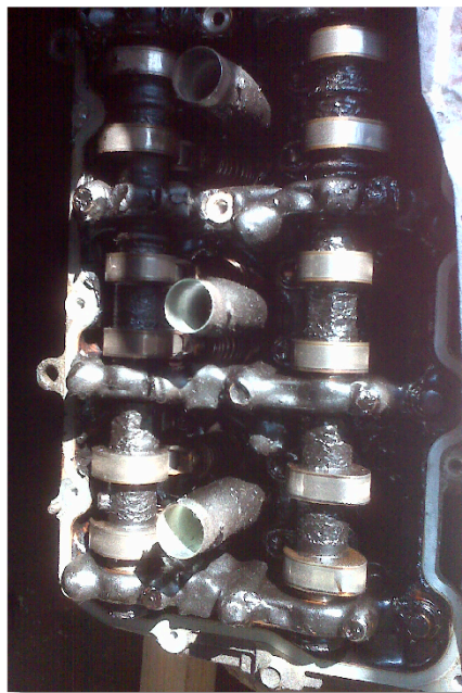
Thick, sludgy oil deposits in the camshaft housing
