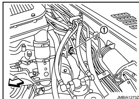
3. Check voltage between CMP sensor terminal 3 and ground with CONSULT-III or tester.
