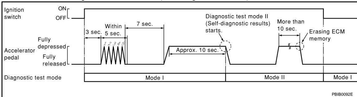
How to Erase Diagnostic Test Mode II (Self-diagnostic Results)
