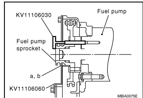
9. Using the extension bar and the TORX socket (size: E10) (commercial service tool), remove the tightening bolts.
