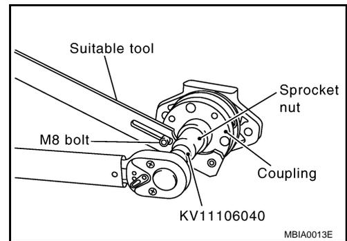
14. Remove coupling with a suitable puller.
