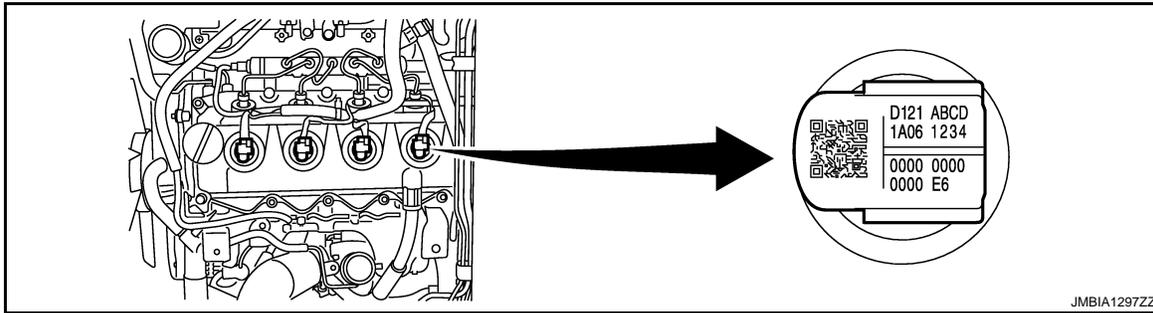
Example: Injector adjustment value = D121ABCD1A061234000000000000E6
