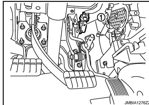
3. Check voltage between APP sensor terminal 4 and ground with CONSULT-III or tester.
