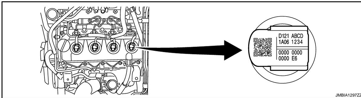
Example: Injector adjustment value = D121ABCD1A061234000000000000E6
