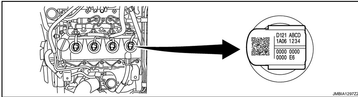
Example: Injector adjustment value = D121ABCD1A061234000000000000E6
