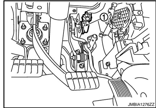
3. Check voltage between APP sensor terminal 6 and ground with CONSULT-III or tester.
