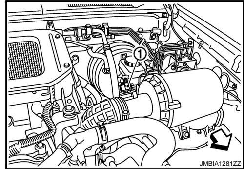
3. Check voltage between mass air flow sensor terminal 2 and ground with CONSULT-III or tester.
