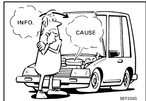
A visual check only may not find the cause of the incidents. A road test with CONSULT-III (or GST) or a circuit tester connected should be performed. Follow the "WORK FLOW".
