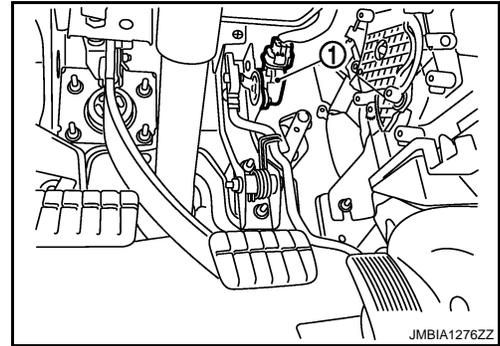
3. Check voltage between APP sensor terminals 4, 6 and ground with CONSULT-III or tester.
