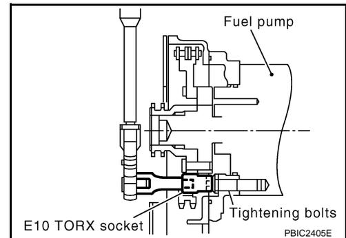
10. Remove the fuel pump toward the rear of engine.
