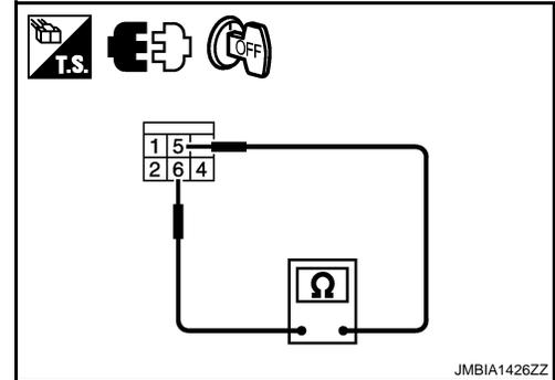
5. Check continuity between heat up switch terminals 4 and 6 under the following conditions.
