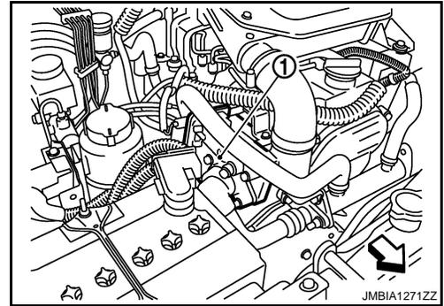
4. Check voltage between EGR volume control valve terminal 3 and ground with CONSULT-III or tester.
