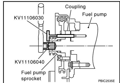
7. Using the hexagonal wrench [SST (KV11106050)] remove tightening bolts of fuel pump sprocket.
