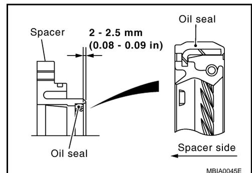
2. Install spacer to fuel pump.
