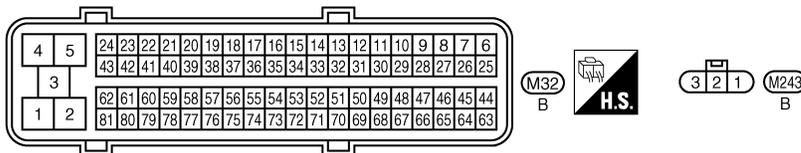
Specification data are reference values and are measured between each terminal and ground.
