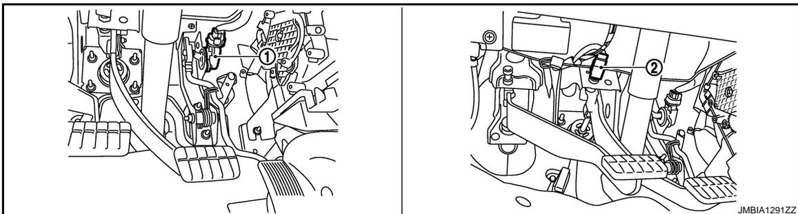
1. Accelerator pedal position sensor
