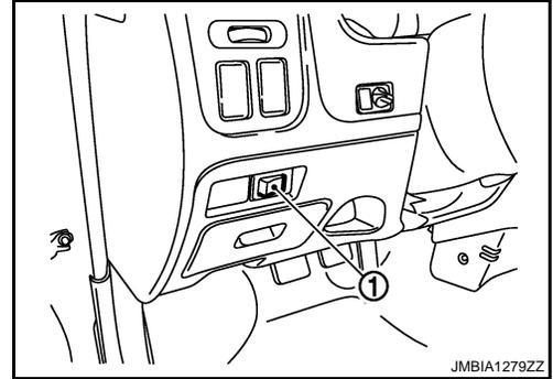
5. Check voltage between heat up switch terminal 6 and ground with CONSULT-III or tester.
