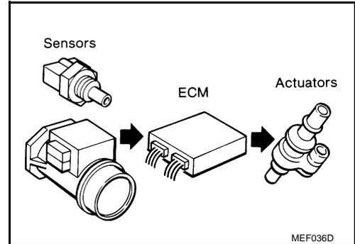
It is much more difficult to diagnose a malfunction that occurs intermittently rather than continuously. Most intermittent malfunctions are caused by poor electric connections or improper wiring. In this case, careful checking of suspected circuits may help prevent the replacement of good parts.
