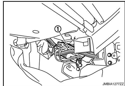
3. When disconnecting ECM harness connector, loosen it with levers as far as they will go as shown in the figure.
