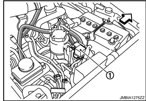
3. Check voltage between ECM relay terminals 1, 3 and ground with CONSULT-III or tester.
